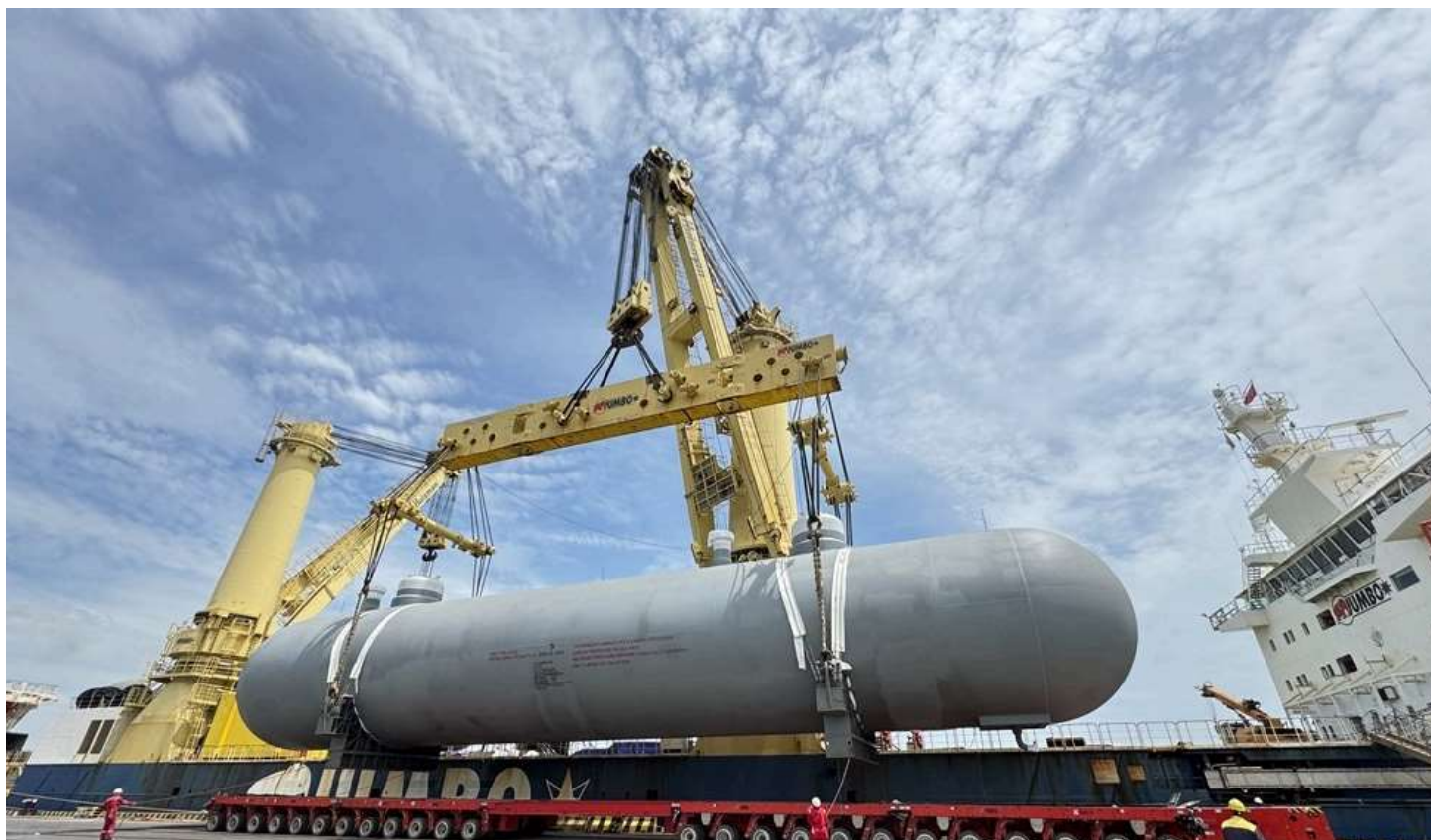
Bullet-shaped tanks are unloaded in Antwerp from a Jumbo Maritime heavy-lift ship. Photo credit: INEOS / Jumbo Maritime.
